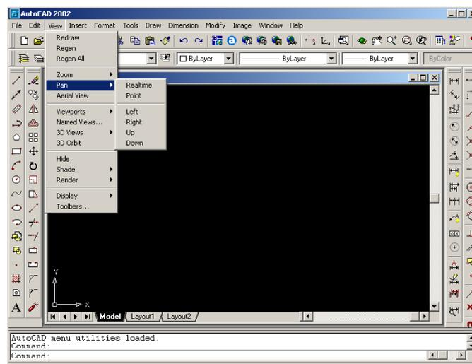
Figure 6: Screen layout for 'pan' command
