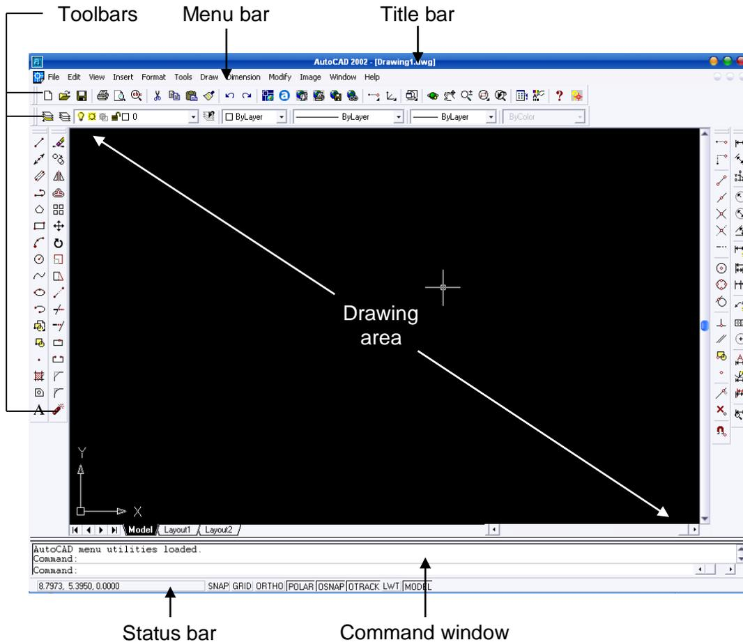
Figure 1: AutoCAD screen layout
